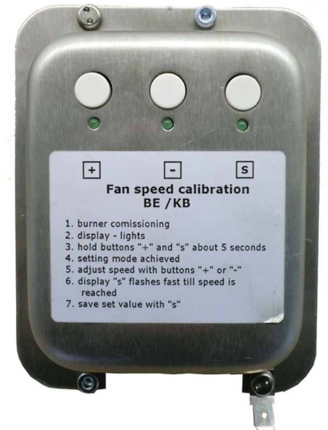
Controller board, with the description of the fan speed adjustment
